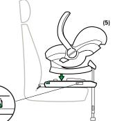
**6-** Move the carrying handle to the 'safe-to-drive' position by pushing the handle release buttons on the inside of the handle. Push the carrying handle towards the vehicle seat as far as possible. There are 2 safe-to drive positions: A and B (6).
