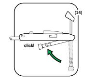
7- Remove the ISOfix insertion clips from the vehicle seat and store them underneath the base (15).
